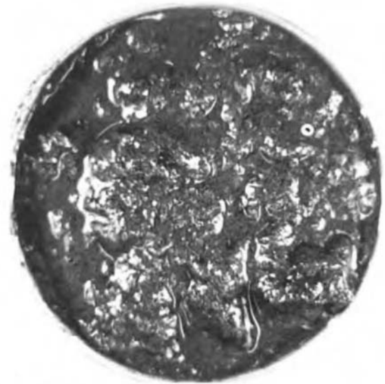
Fig. 3 Flask-shaped pit
