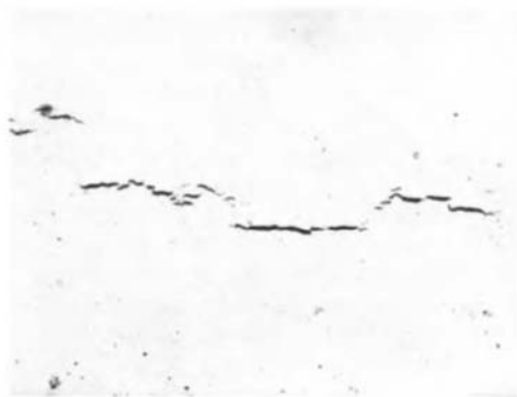
Fig. 1 Hydrogen-induced cracking in a linepipe steel. 30x
