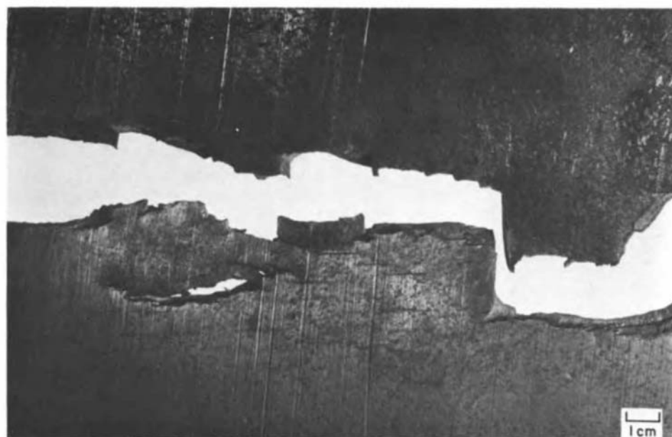
Fig. 3 Secondary cracking in pipe surface adjacent to stress-corrosion cracks shown in Fig. 2. Actual size. See also Fig. 4 and 5.
