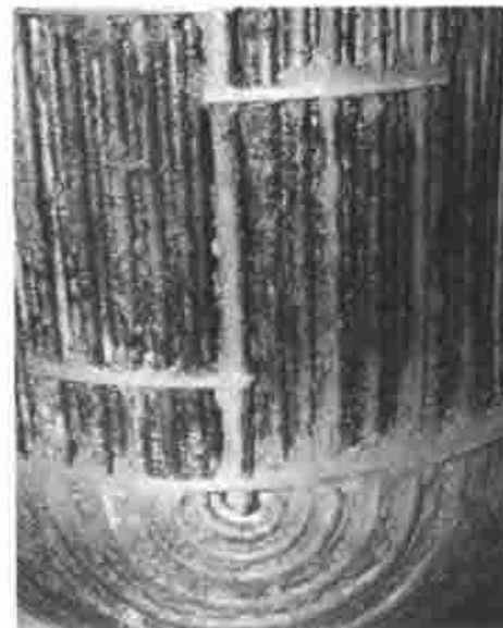
Fig. 5 Fouled heat-exchanger tube bundle
